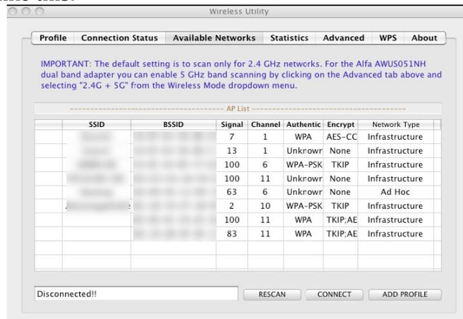
By default, the utility is set to only scan in the 2.4 GHz band network.
