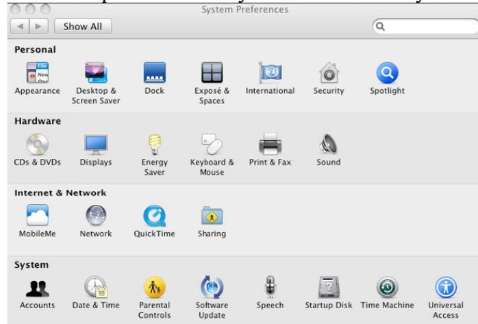
Inside System Preferences, double-click the Network icon. On the left-hand side of the Network window, locate the device called USB Ethernet Adapter (en1) it may be abbreviated as USB...eth. If you have previously installed a wireless USB adapter on your Mac, the item may have a different number at the end.
